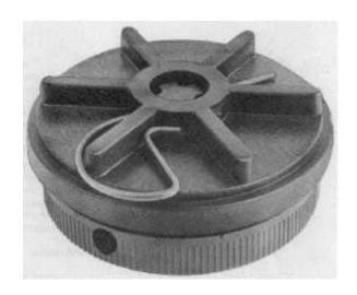
The PRB M409 is a plastic-bodied, circular antipersonnel mine. The fuze is a double percussion type with two opposing steel firing pins. The strikers are held apart by a sliding bolt attached to the pressure plate. The bolt has an aperture holding two percussion caps. When the bolt is displaced, the strikers are released and detonate the percussion caps. The only metal components are firing pins and two aluminum primer caps.
